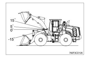
In order to recheck weight, go to the (b) after changing boom position (below -15°).
