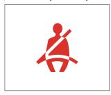
① This lamp lights ON for the first five seconds after starting the engine.
