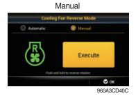
· Manual: Rotate the fan with reverse direction while pressing the button "Execute".
