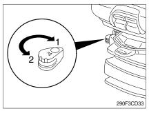
① The absorber setting of the seat can be varied to suit the on and off-road working conditions.
